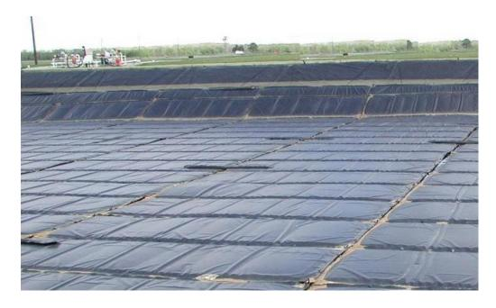
During winter months it can expensive and difficult to keep water from freezing for use in hydraulic fracturing procedures. Heating costs can be dramatically decreased by the use of insulating floating covers to help prevent heat loss of the open body of water. Whether your application is a lined earthen pit of an aboveground steel water tank, Contain Enviro can custom suit your requirements.
